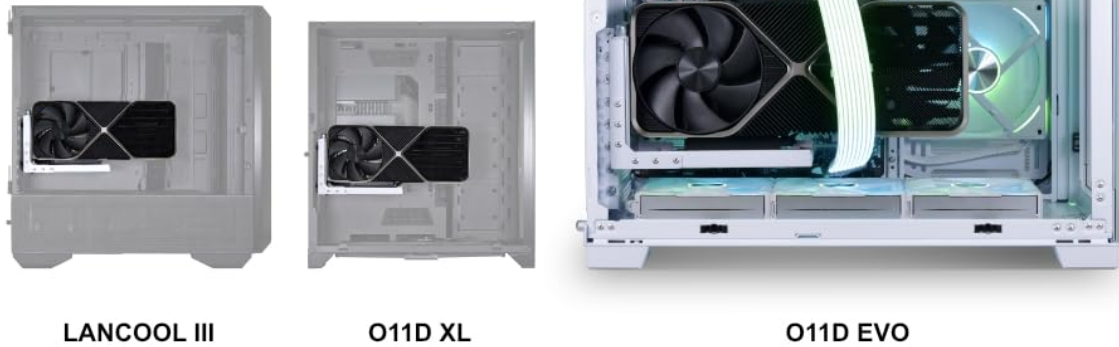
Image 3.1: Visual representation of the vertical GPU kit's compatibility with different ATX cases, such as LANCOOL III, O11D XL, and O11D EVO.
