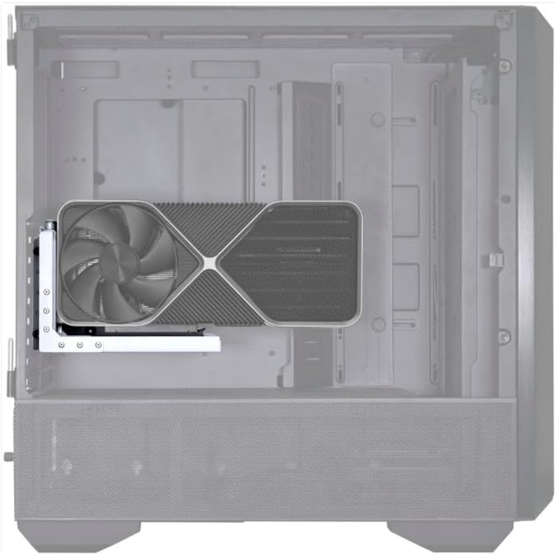
Image 3.3: Illustrative diagram of a graphics card vertically mounted inside a computer case, highlighting the position and orientation.
