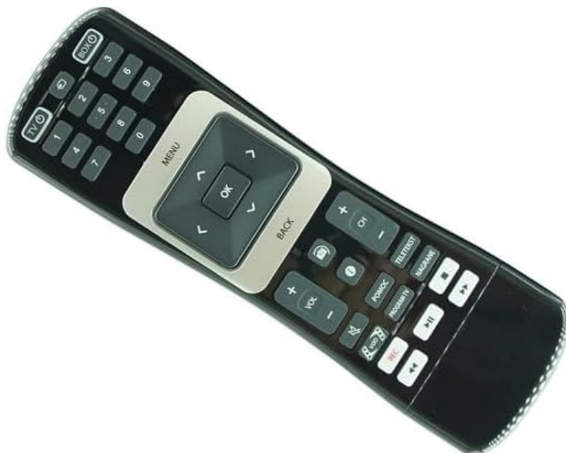
Figure 2.1: Front view of the remote control. This side features a numeric keypad (0-9), channel and volume controls, menu navigation buttons (OK, arrow keys, MENU, BACK), and media playback buttons (play, pause, stop, fast forward, rewind, record).
