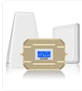
Figure 3: Key features of the GAGBK Cell Signal Booster, including LCD, AGC, ALC, self-oscillation, sleep mode, and aluminum alloy construction.
