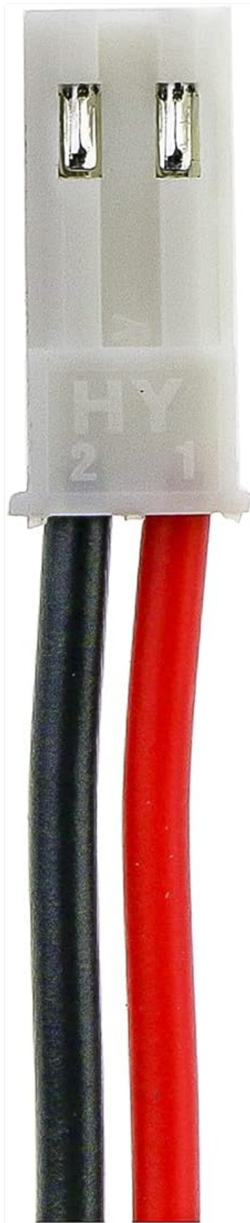
Image 3.2: A detailed view of the battery's connector, highlighting the two-pin design for proper connection.
