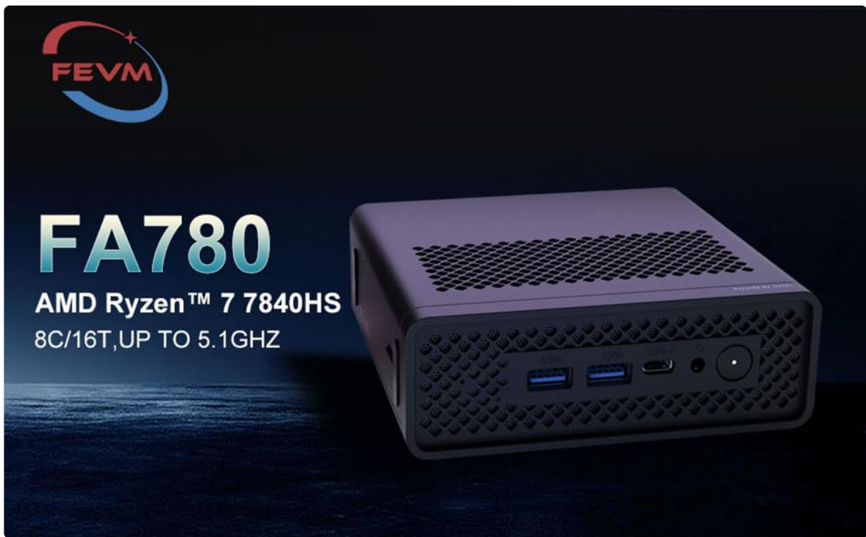
Figure 3.1: The FEVM FA780 Mini PC is significantly smaller than a standard desktop computer, with dimensions of approximately 1.73in (height) x 4.96in (width) x 4.49in (depth).
