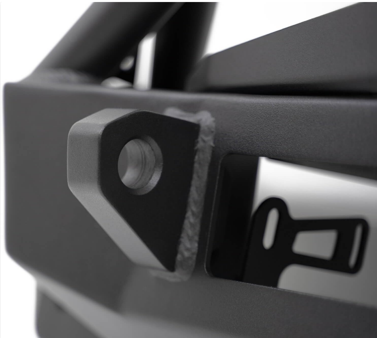
Image: A close-up shot of the D-ring mount on the DV8 Offroad FS-1 Series Stubby Front Bumper, illustrating its solid construction and weld points.
