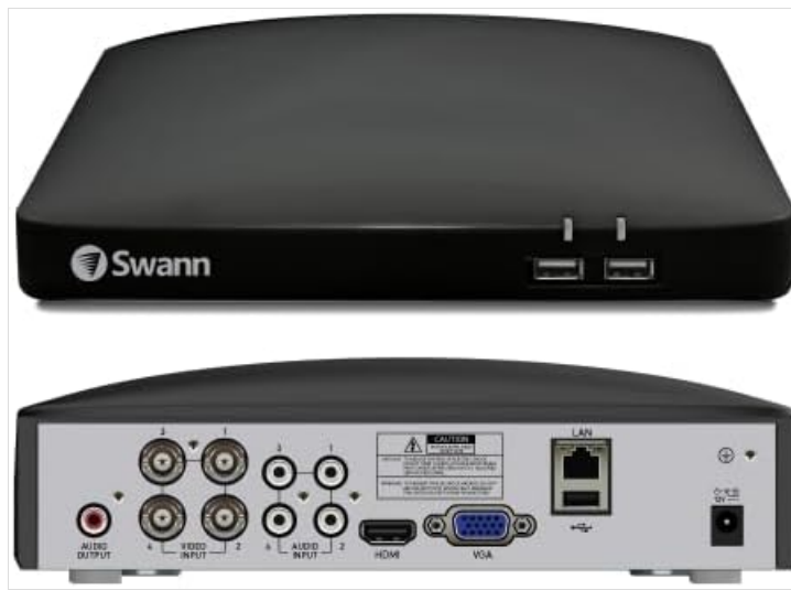
Figure 2: Rear panel of the Swann DVR4-4685 DVR, illustrating BNC video inputs (1-4), RCA audio inputs (1-4), RCA audio output, HDMI output, VGA output, LAN port, USB ports, Micro SD card slot, and power input.
