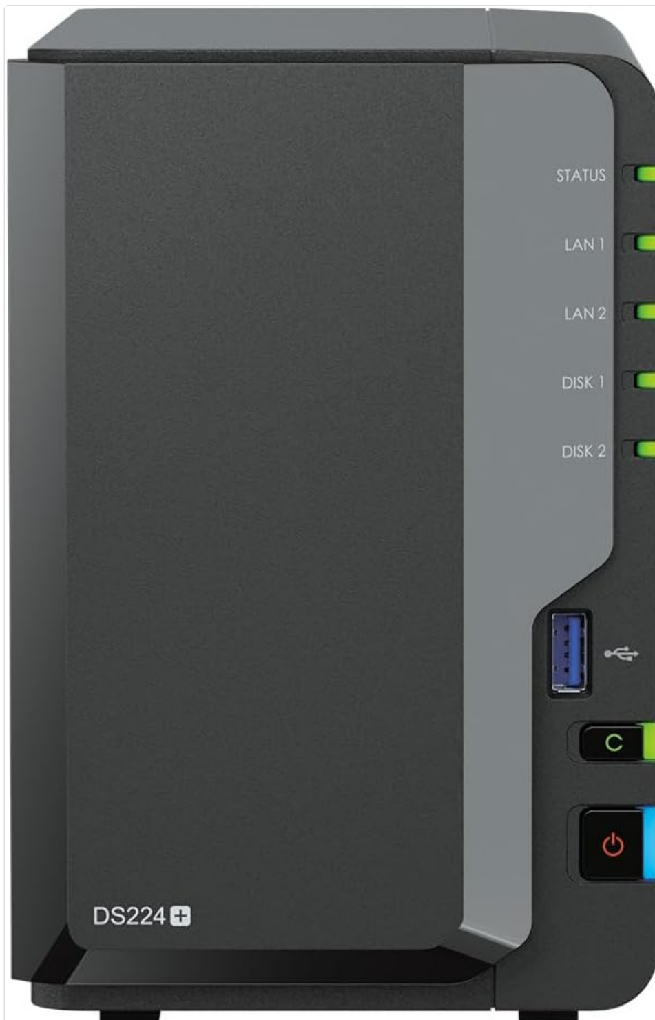
Figure 1: Front view of the Synology DS224+ NAS, showing the power button, USB port, and status indicator lights for system, LAN, and disks.
