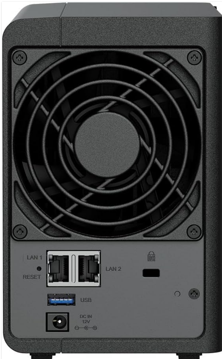
Figure 2: Rear view of the Synology DS224+ NAS, highlighting the two RJ-45 1GbE LAN ports and USB 3.2 Gen 1 ports for network and peripheral connections.
