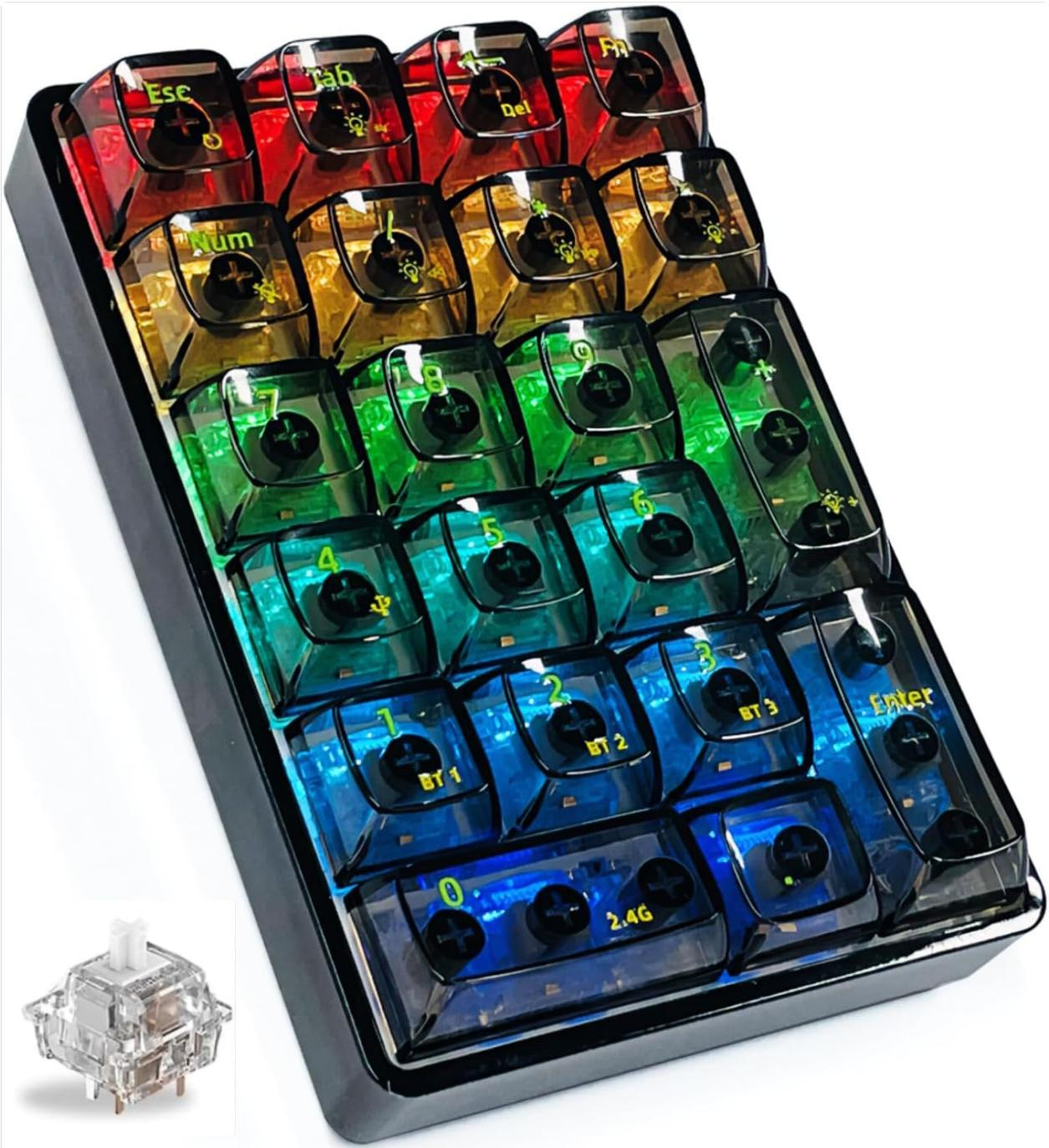
A clear view of the SOLAKAKA K21 number pad, highlighting its transparent keycaps and vibrant RGB backlighting. An individual ice crystal switch is displayed in the bottom left corner.
