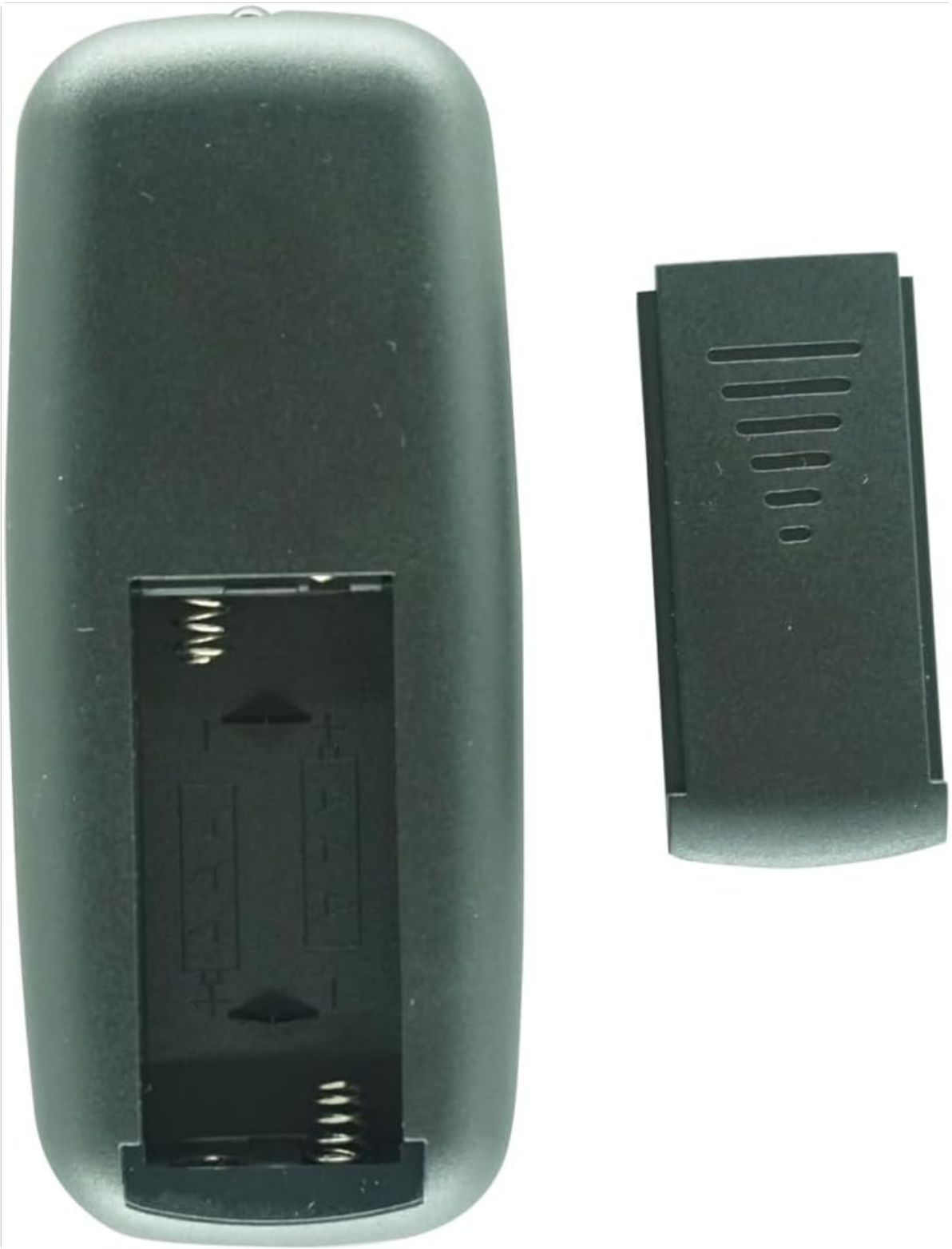
Image: Rear view of the remote control with the battery cover removed, illustrating the correct orientation for inserting two AAA batteries.
