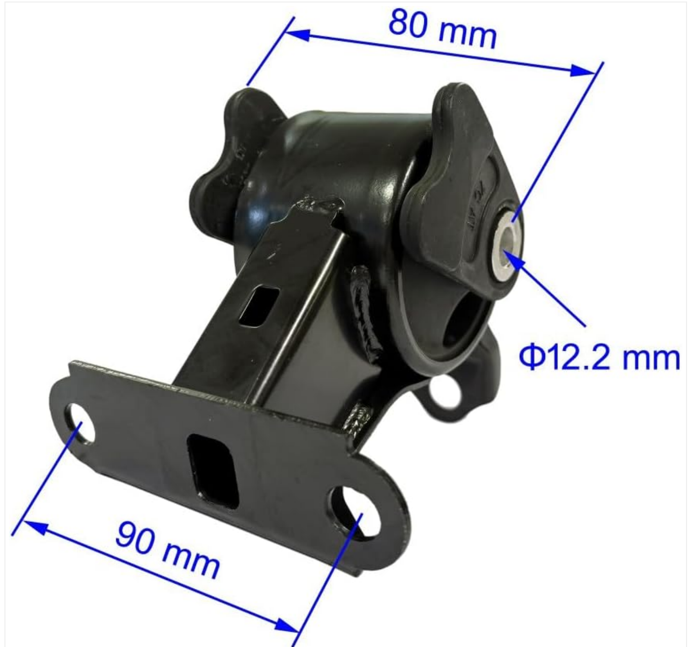
Image 4.4: Detailed dimensions of the Front Right Motor Mount (A4503, A4567).
