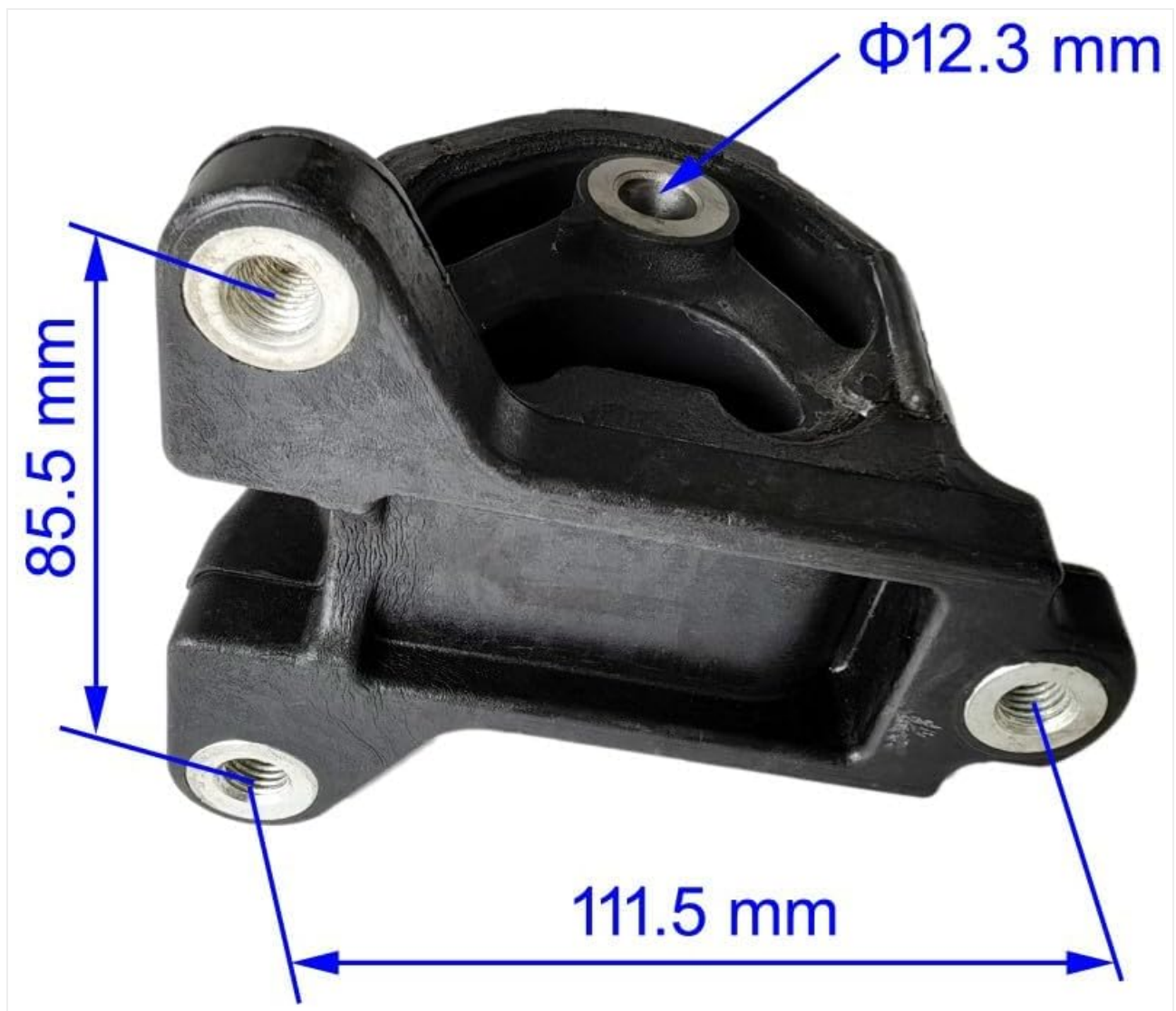
Image 4.3: Detailed dimensions of the Transmission Mount (A4506, A4579, A4545).
