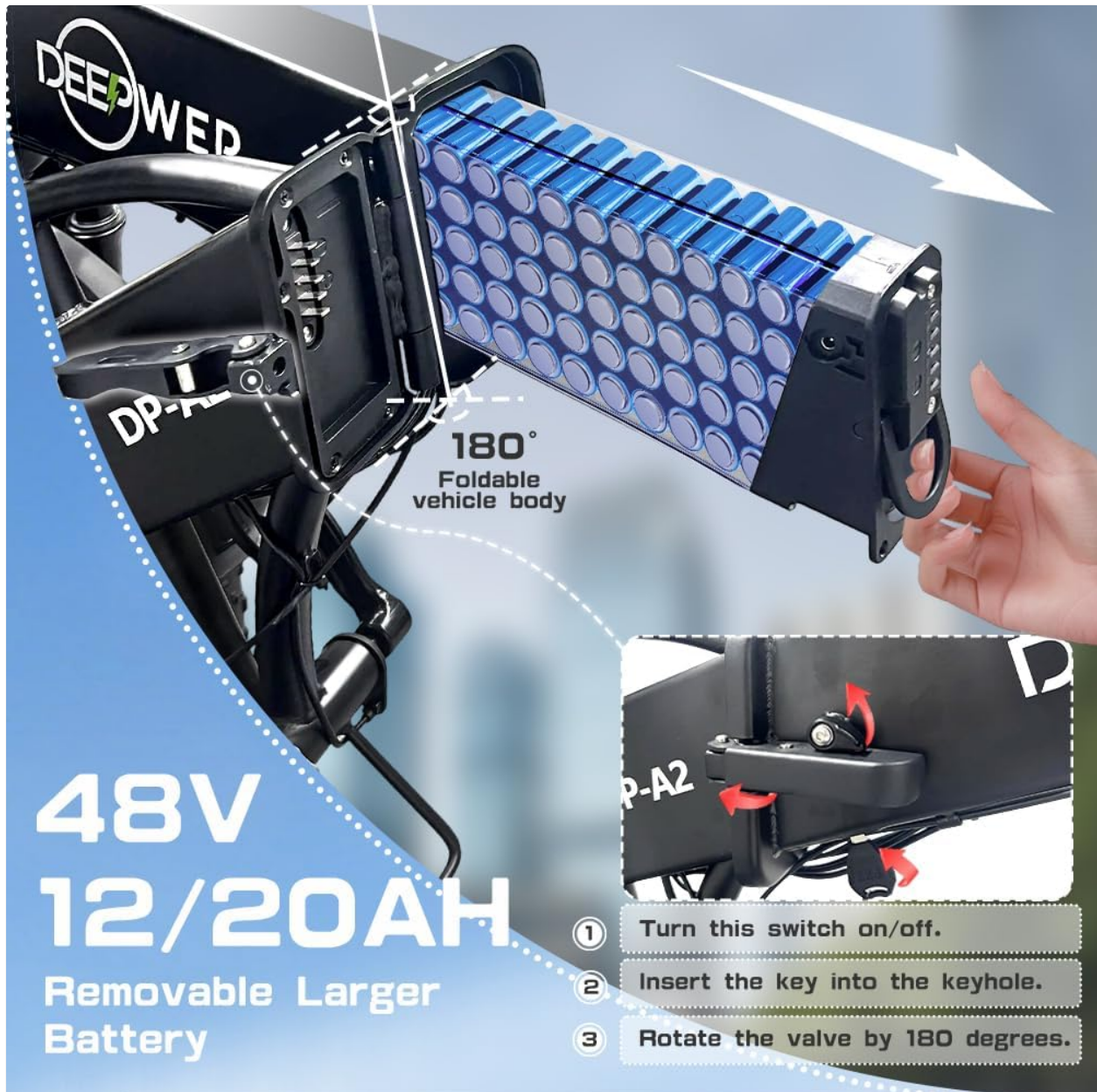
Figure 5.1: Removable 48V 20Ah battery.
