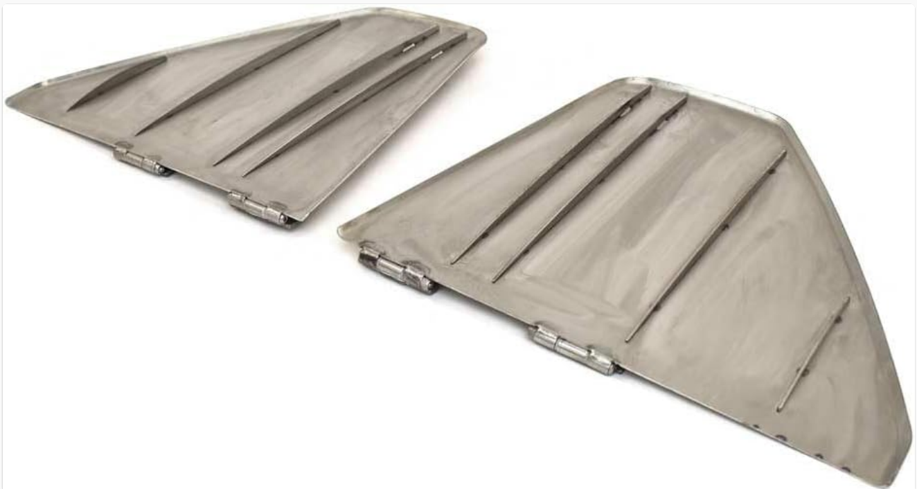
Figure 4.2: The underside of the trim tabs, revealing the structural ribs that provide rigidity and the attachment points for the hinges. This view is important for understanding the mounting surface.
