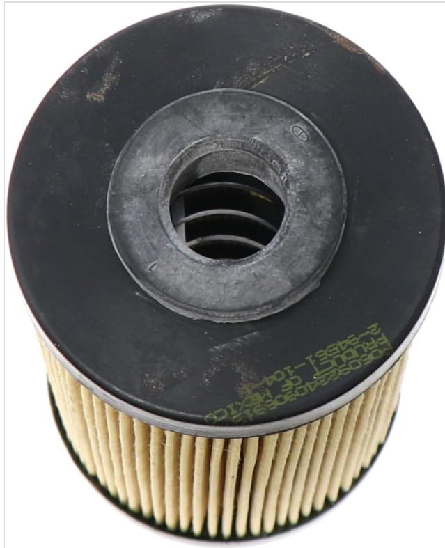
Figure 7.1: Top view of the fuel filter, showing the inlet/outlet port.
