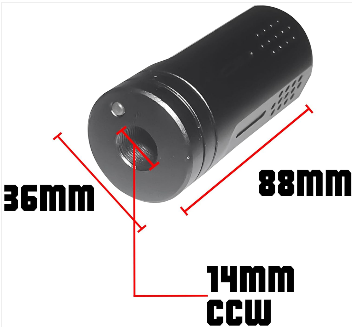
Image: A diagram illustrating the key dimensions of the tracer unit, including its length (88mm), diameter (36mm), and 14mm CCW thread interface.
