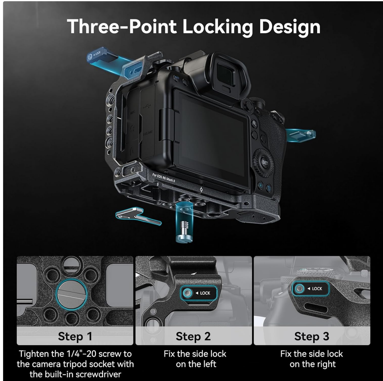
Figure 4.1: Three-Point Locking Design installation steps.
