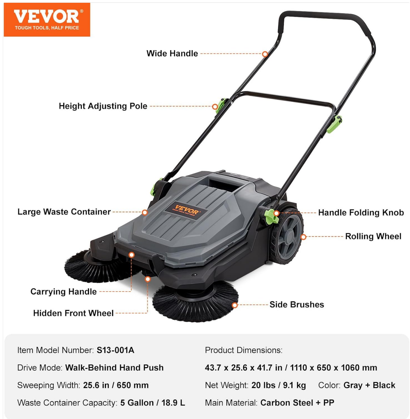
Figure 2: A detailed diagram labeling all major components of the sweeper.
