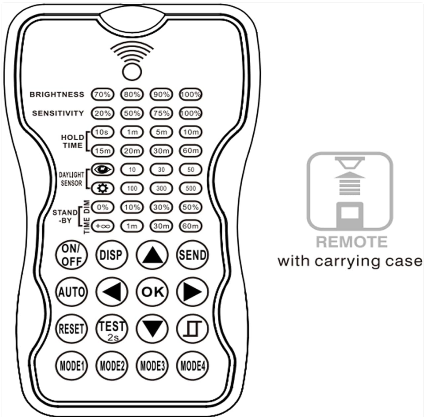
Figure 2: Diagram of the RC-100 remote control, illustrating its layout and indicating it comes with a carrying case.
