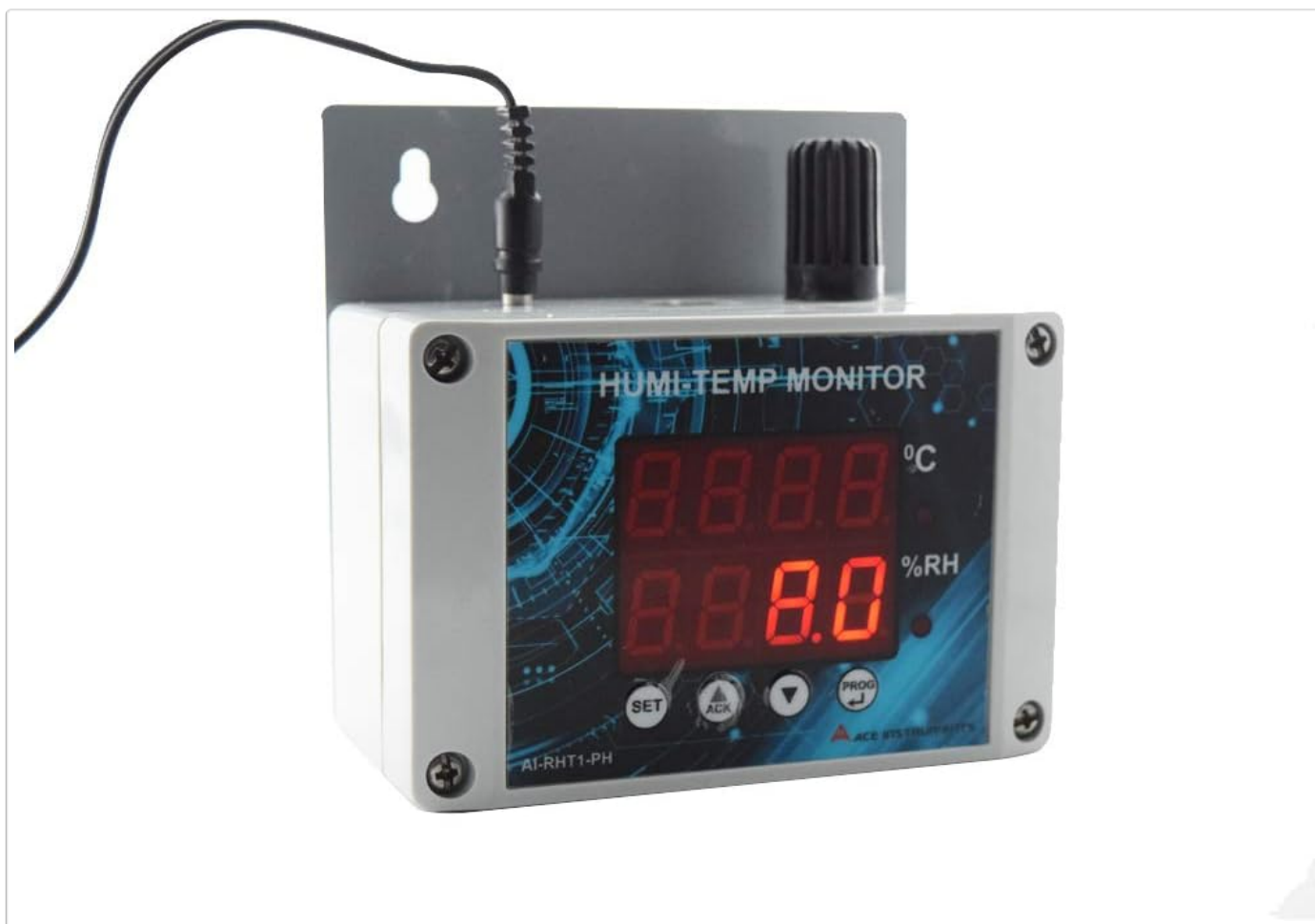
Figure 3: Side view of the monitor, illustrating the wall mounting bracket and various connection ports.
