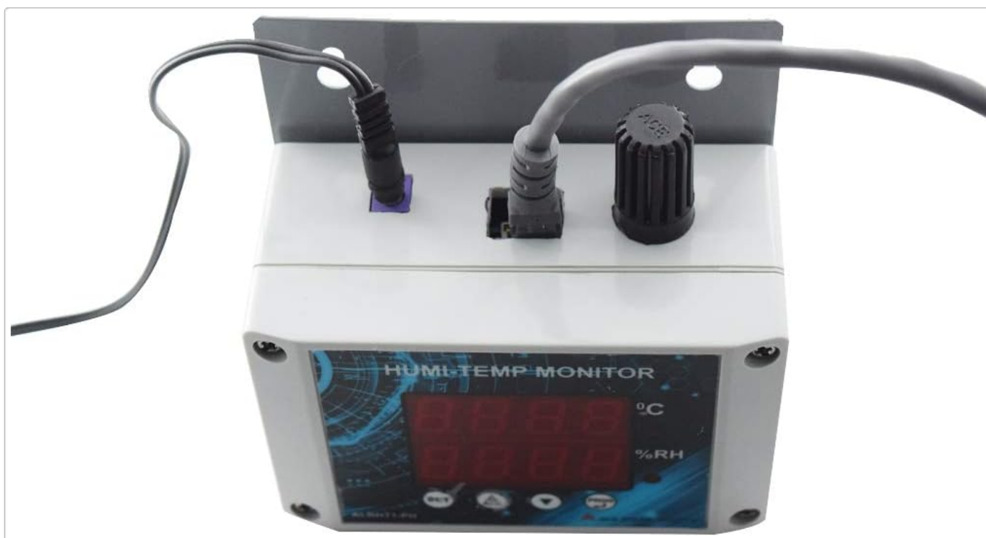
Figure 4: The monitor connected with an optional external probe for flexible sensor placement.
