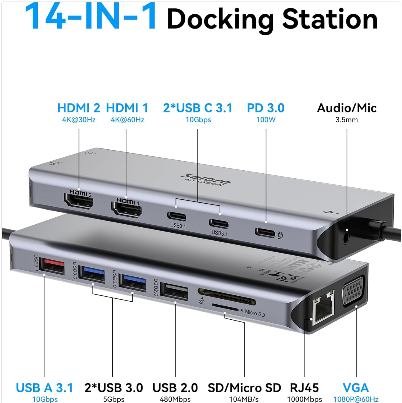
Image 3.1: Detailed view of the docking station's ports and their specifications.
