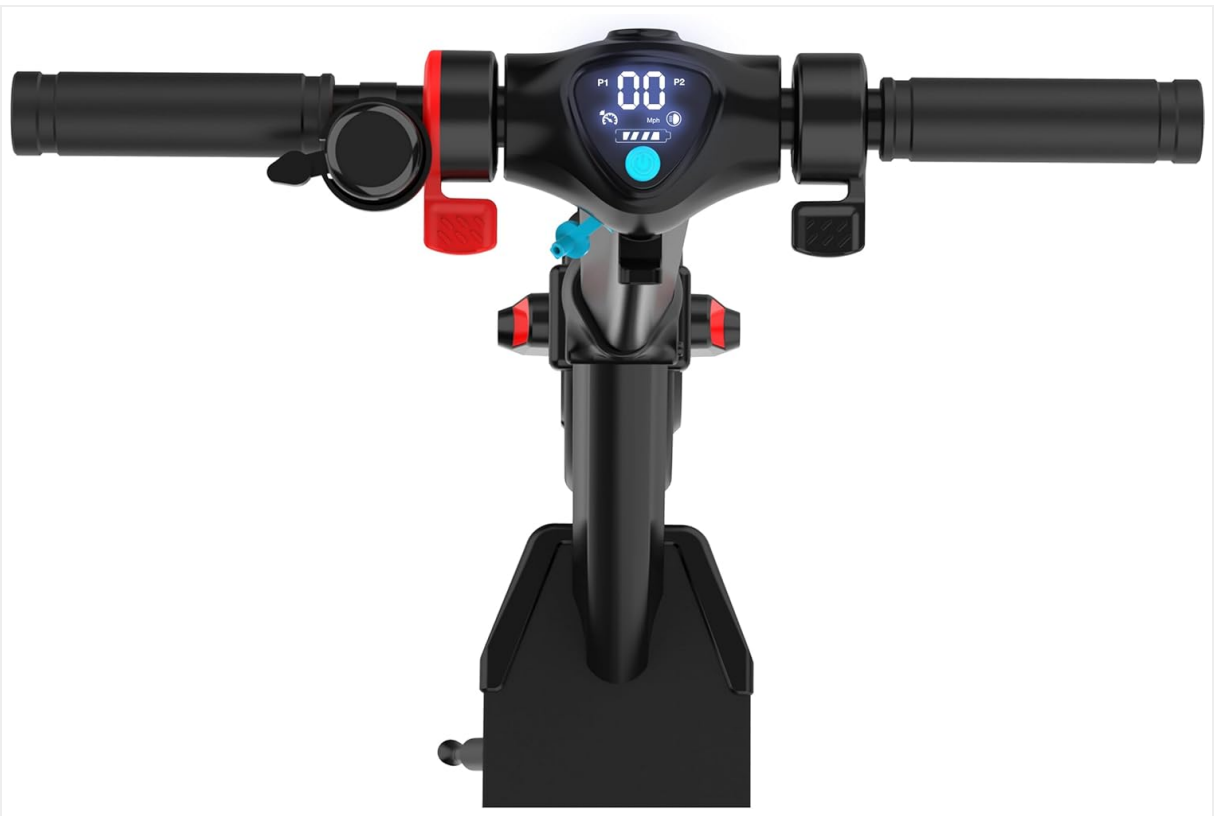
Figure 4.2: Close-up of the scooter's handlebars, showing the LCD digital display, throttle, and brake levers for intuitive control.
