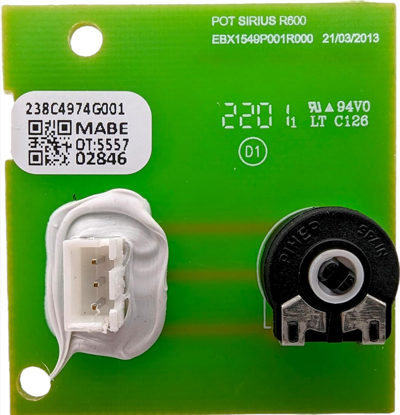
Figure 1: Front view of the Mabe Refrigerator Control Board. This image displays the main components including the white multi-pin connector, a black potentiometer, and various circuit traces. The board is green with white markings indicating part numbers
