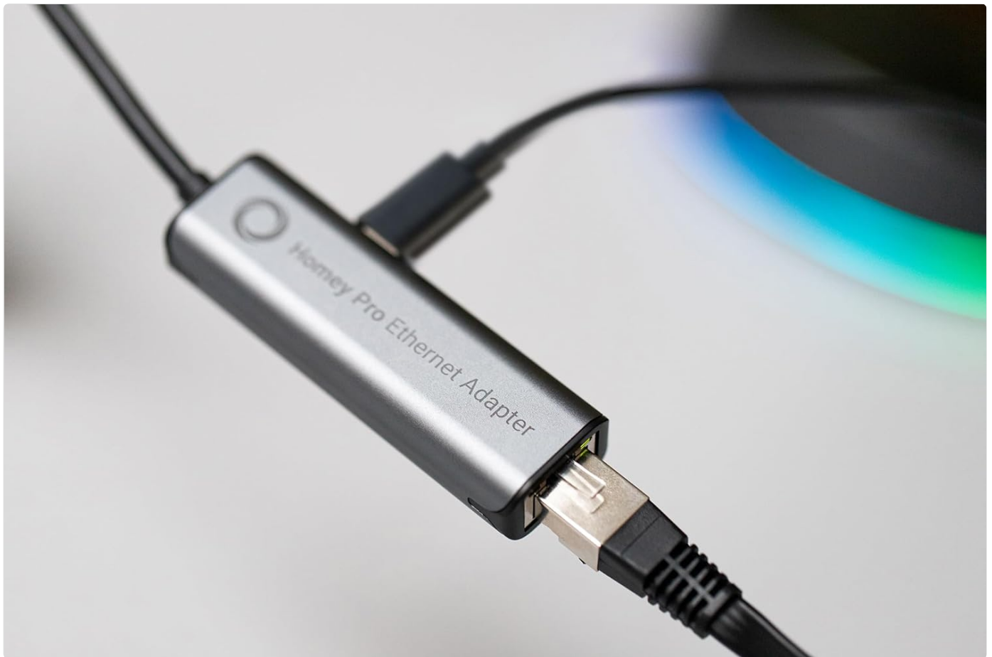
Image: A close-up view of the Homey Pro Ethernet Adapter successfully connected and in use with the Homey Pro device, showing the Ethernet cable plugged in.
