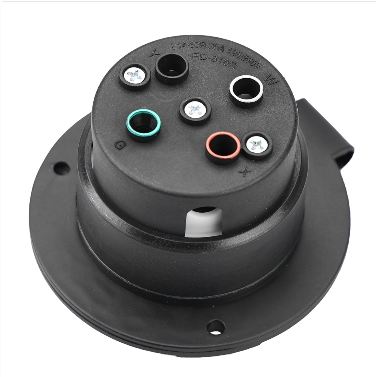
Image: Rear view of the L14-30R outlet, displaying the four color-coded terminals for wiring connections (Green for Ground, White for Neutral, Red and Black for Hot).
