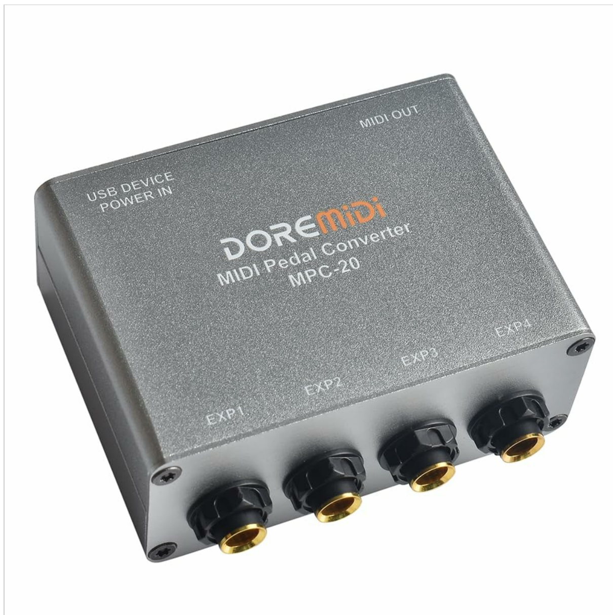
Figure 1: Top-down view of the DOREMiDi MPC-20 MIDI Pedal Converter. This image highlights the USB DEVICE POWER IN port, MIDI OUT port, and the four expression pedal input jacks labeled EXP1, EXP2, EXP3, and EXP4.
