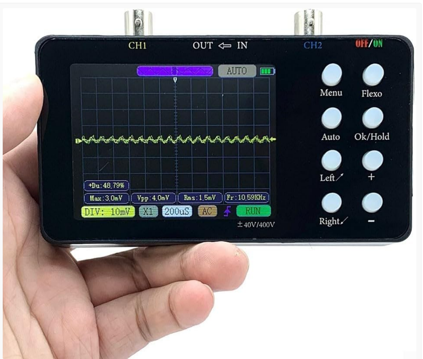
Front view of the SCO2 Oscilloscope, showing the display, input channels (CH1, CH2), output, input, and control buttons.
