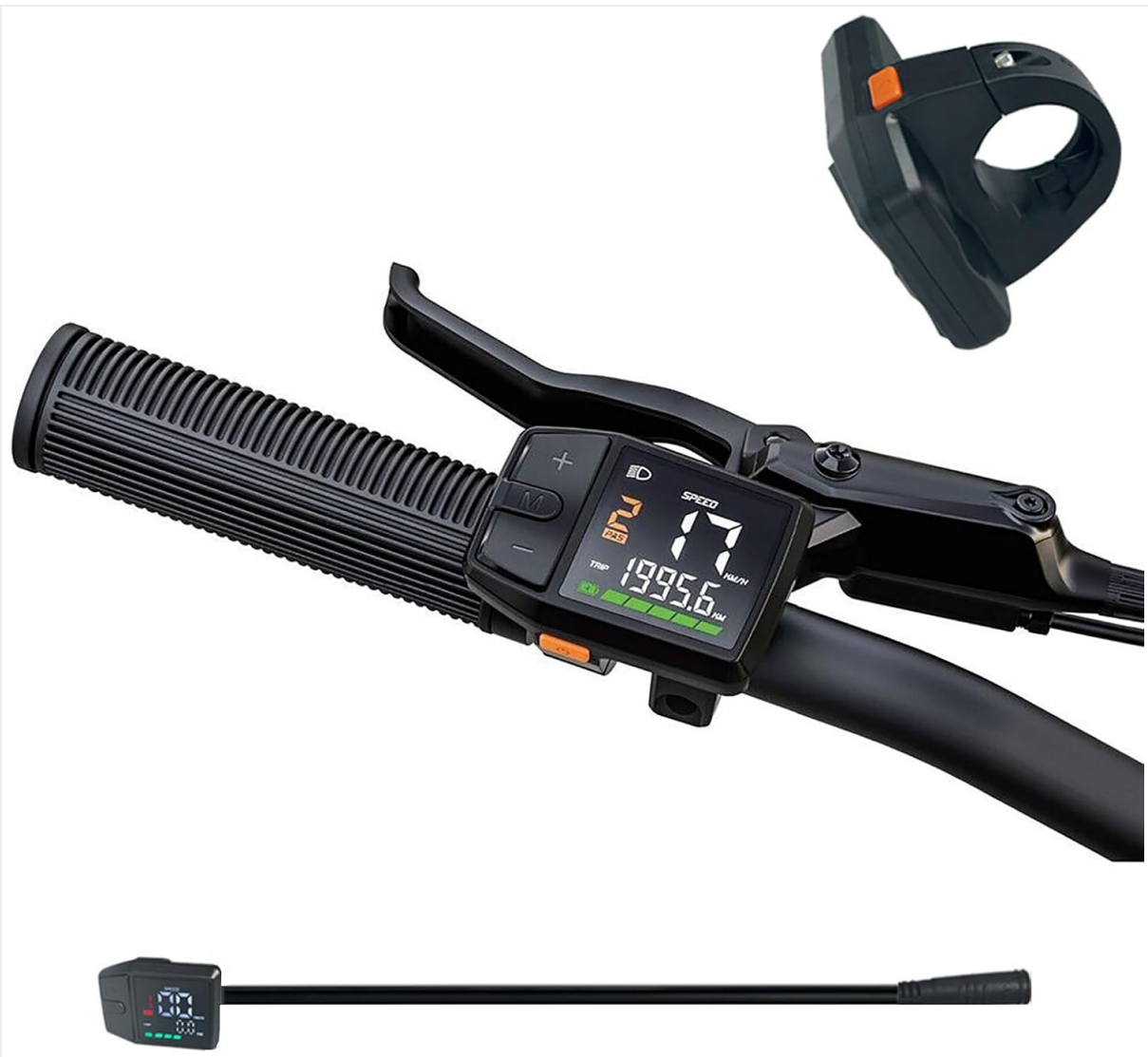
Figure 4.1: Overall view of the DZ41 LCD Display Meter mounted on an e-bike handlebar, showing the display unit and a separate remote button unit.
