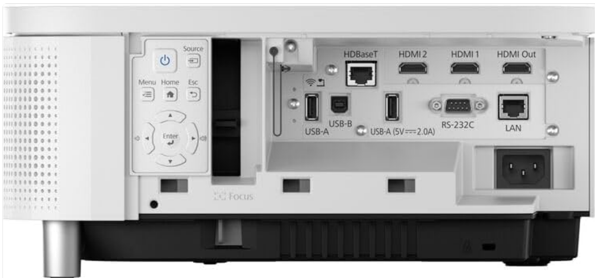
Figure 3: Rear panel of the projector, displaying various input and output ports including HDMI, USB, LAN, and RS-232.
