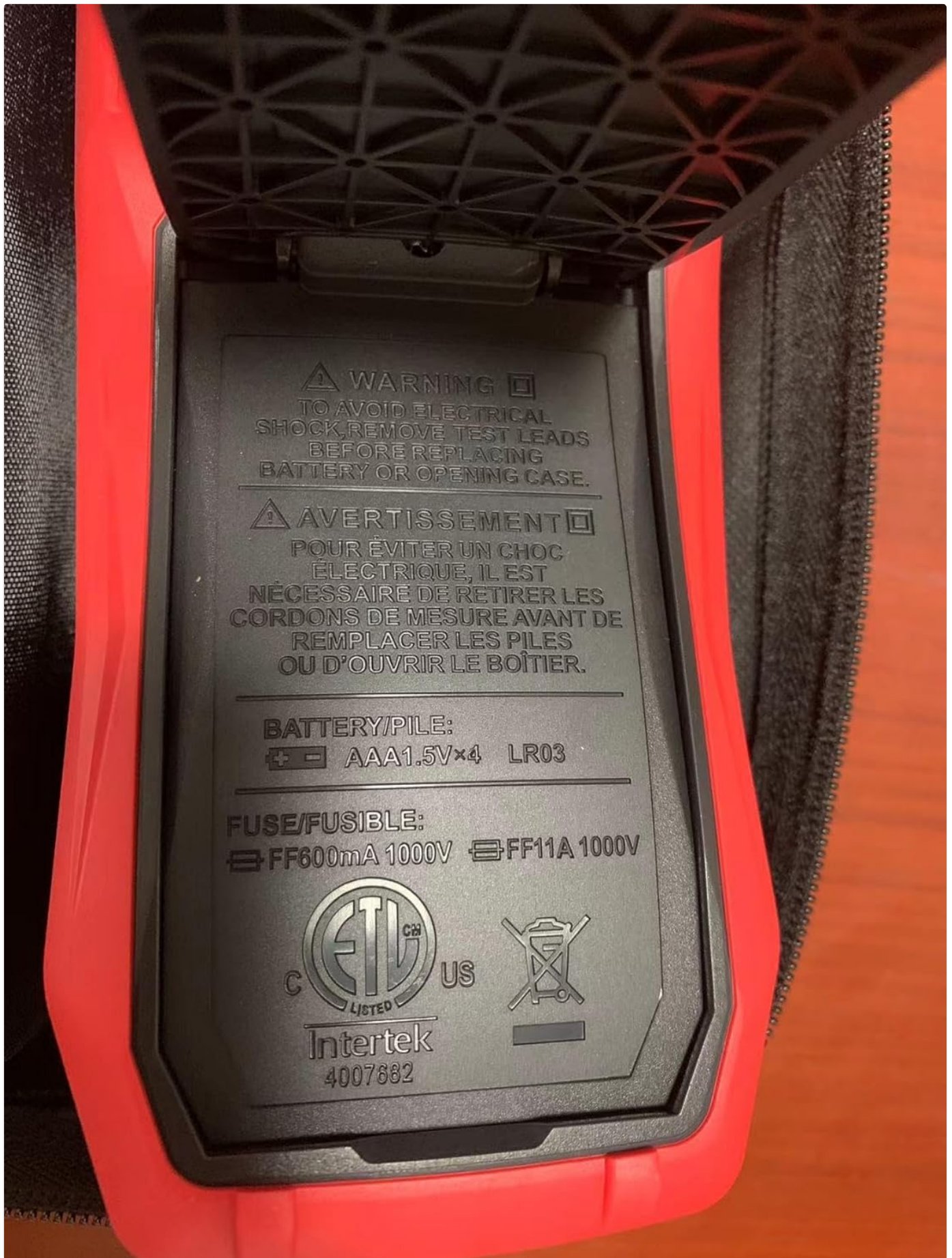
Figure 3: View of the battery compartment, showing battery type (AAA 1.5V x 4) and fuse specifications (FF600mA 1000V, FF11A 1000V).
