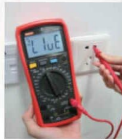
Live and nature wires identification
