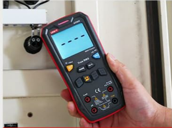
Non-contact electrical testing
