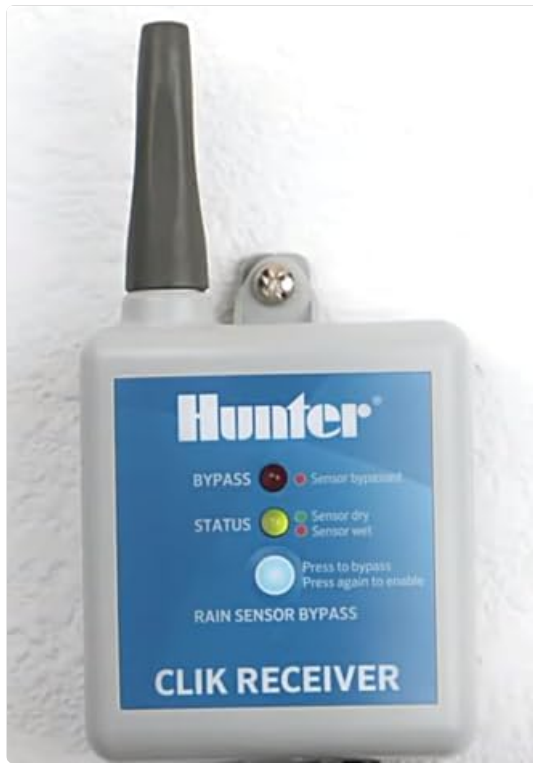
Figure 3: Hunter CLIK RECEIVER Unit. This image displays the receiver unit with its antenna, status indicator lights (Bypass, Status), and a button for rain sensor bypass.
