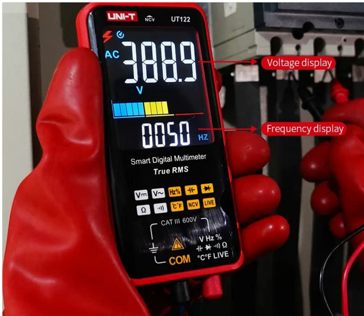
Figure 5.3: Voltage and Frequency Display. The multimeter can simultaneously display voltage and frequency, as shown here with AC 388.9V and 50Hz.
