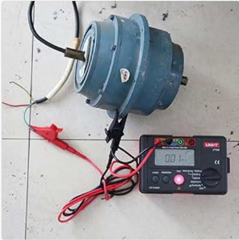
Figure 7: UT526 connected for ground resistance testing.
