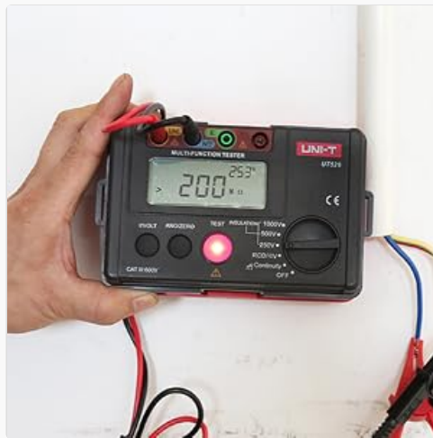
Figure 6: UT526 performing a low resistance continuity test on a motor.
