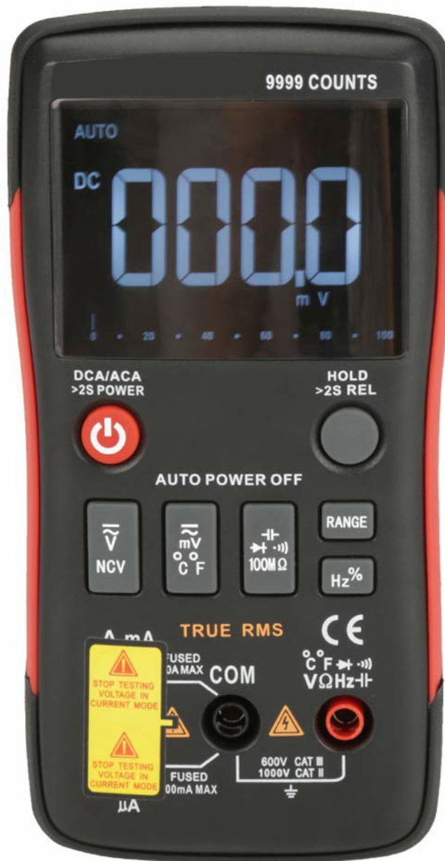
Image 4.1: Front panel detailing input jacks and function buttons.
