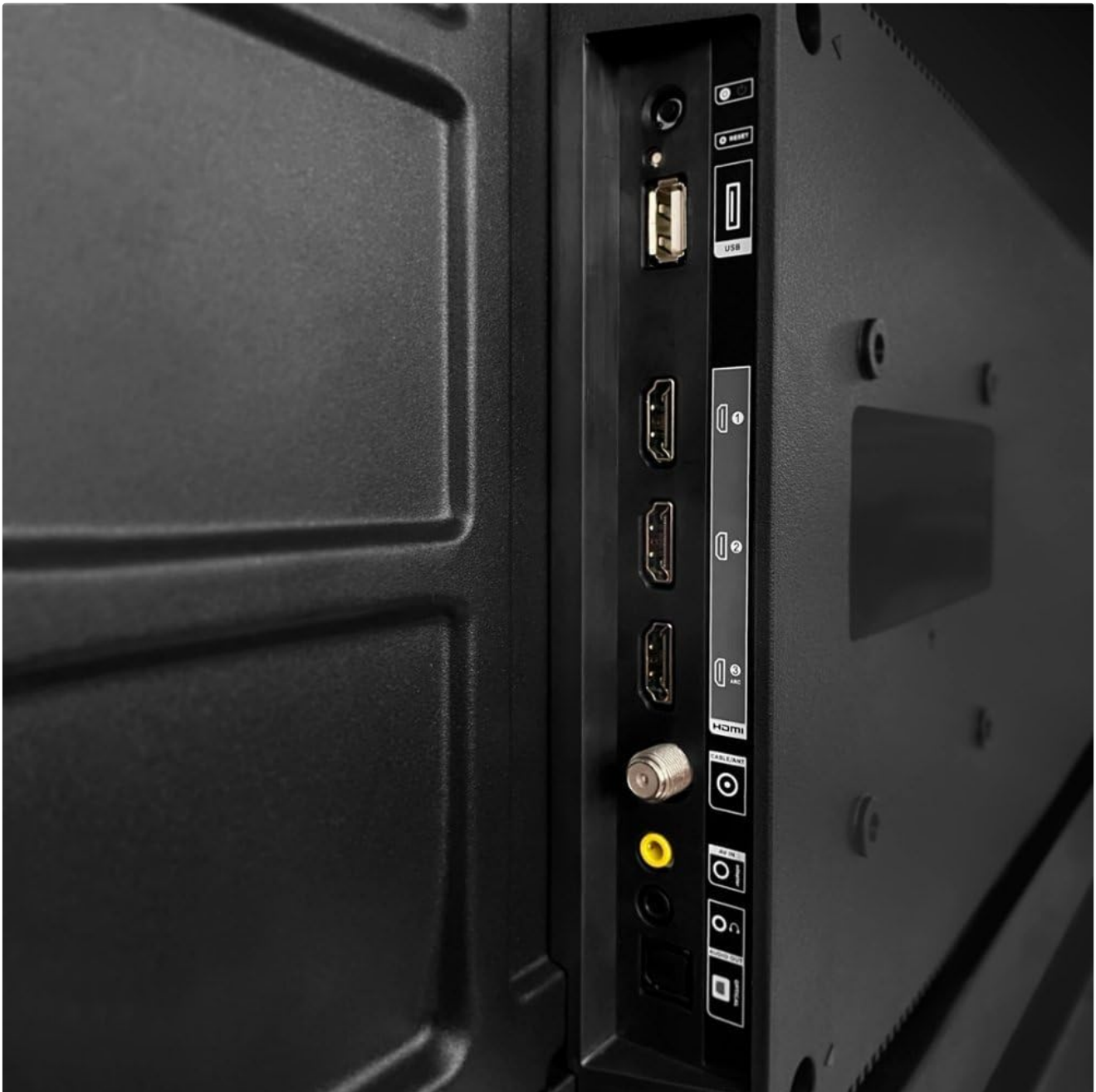
Figure 5.1: Side view of the TV's input ports.
