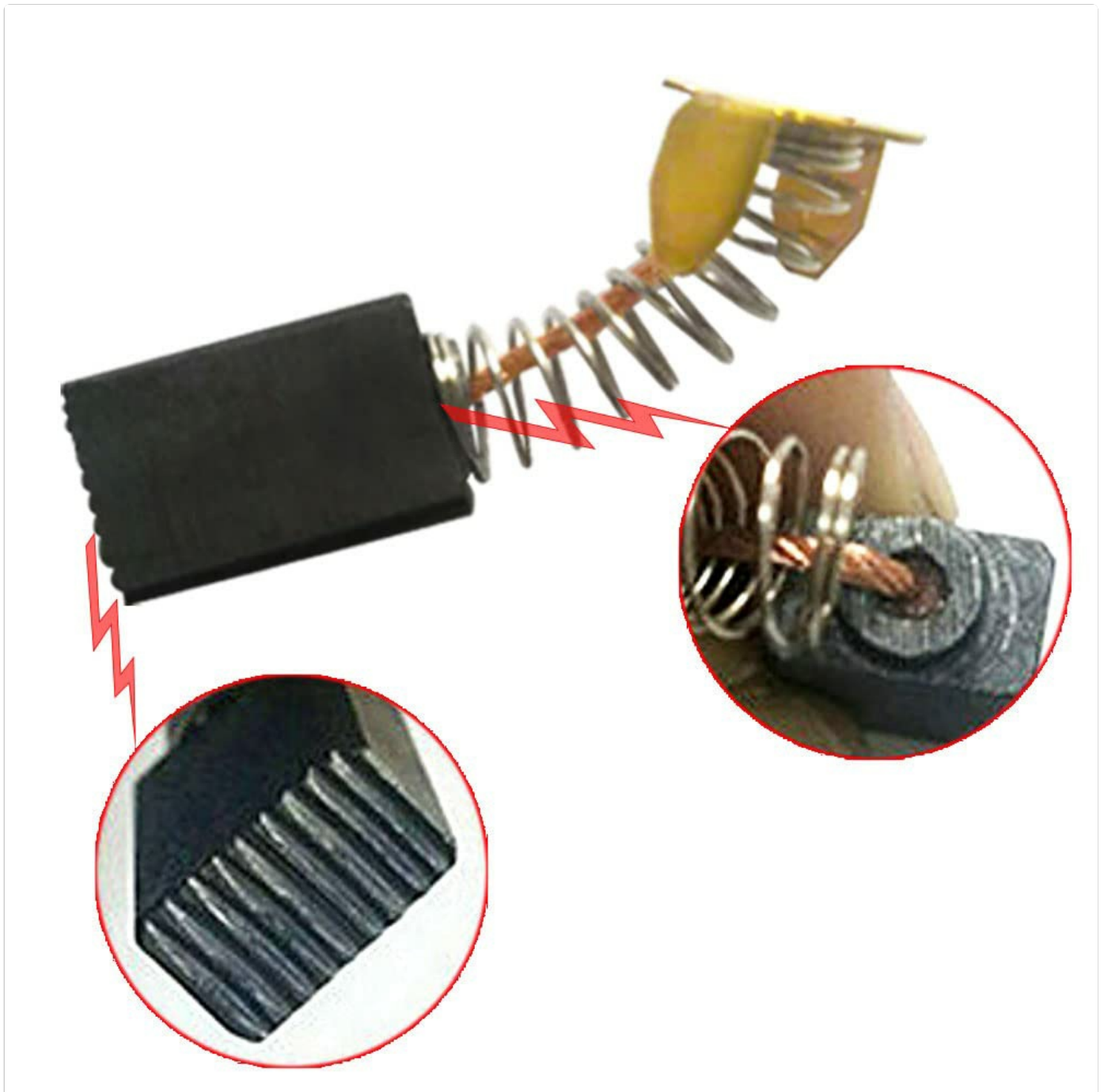
Image: A magnified view of a single carbon brush, highlighting its key components: the solid carbon block, the coiled spring that provides tension, and the copper wire connecting it to the motor's electrical system.
