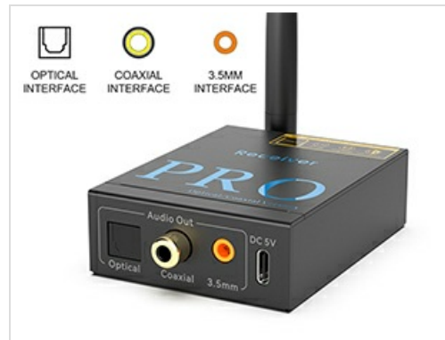
Image: The receiver unit of the 1Mii RT5066Pro, showing its audio output ports (Optical, Coaxial, 3.5mm) and power input.
