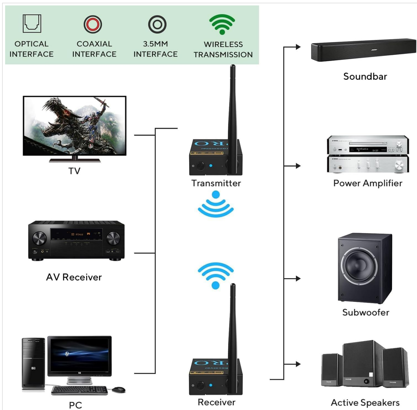
Image: A comprehensive diagram illustrating various input sources (TV, AV Receiver, PC) connected to the transmitter, and various output devices (Soundbar, Power Amplifier, Subwoofer, Active Speakers) connected to the receiver, highlighting Optical, Coaxial, and 3.5mm interfaces.
