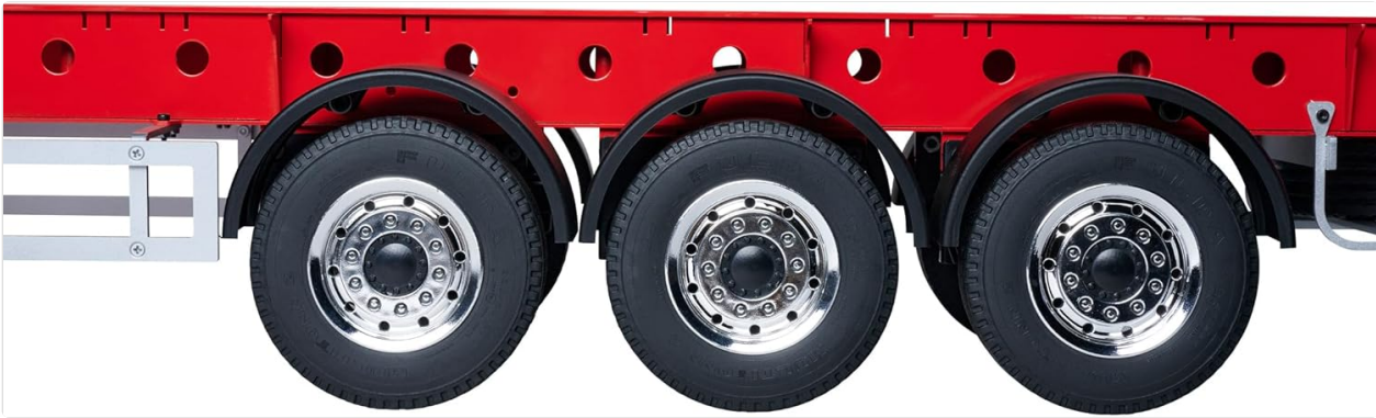
Figure 5: Detail of the three axles, wheels, and mudguards, emphasizing areas for regular inspection and cleaning.
