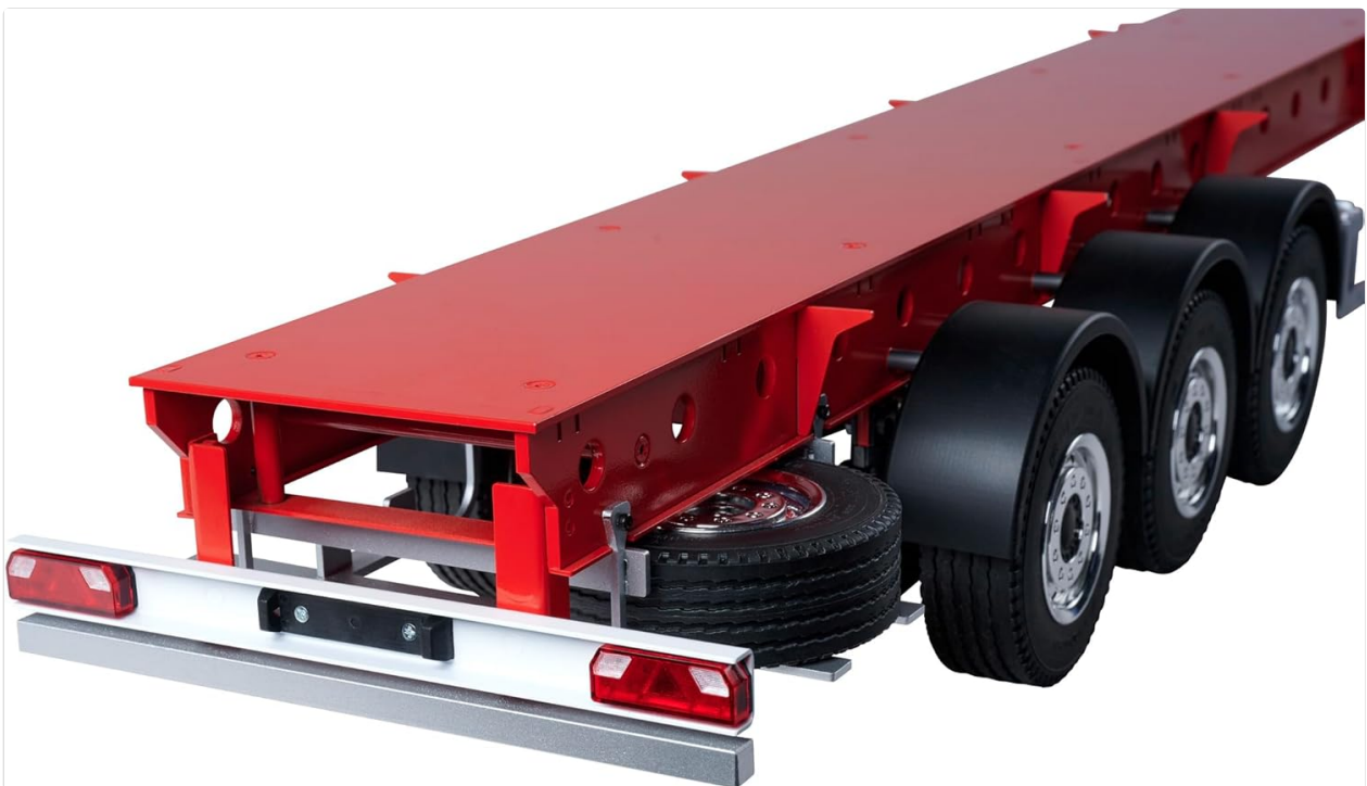
Figure 4: Rear view of the chassis, illustrating the aluminum bumper with 7-chamber rear lights and the spare wheel holder.
