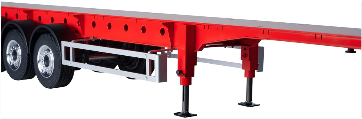
Figure 3: Detail of the adjustable support legs, crucial for stable parking and coupling.
