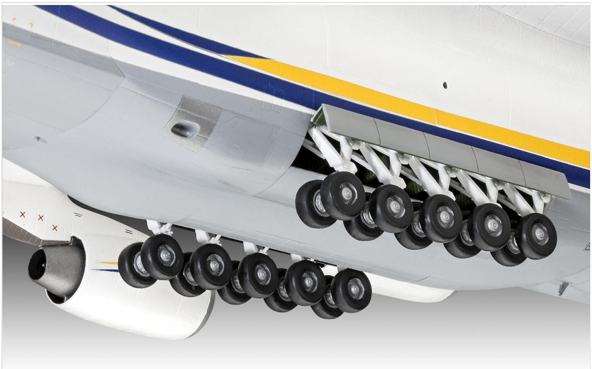
Image 4.3: A close-up of the complex multi-wheel landing gear system on the Antonov An-124 Ruslan model.
