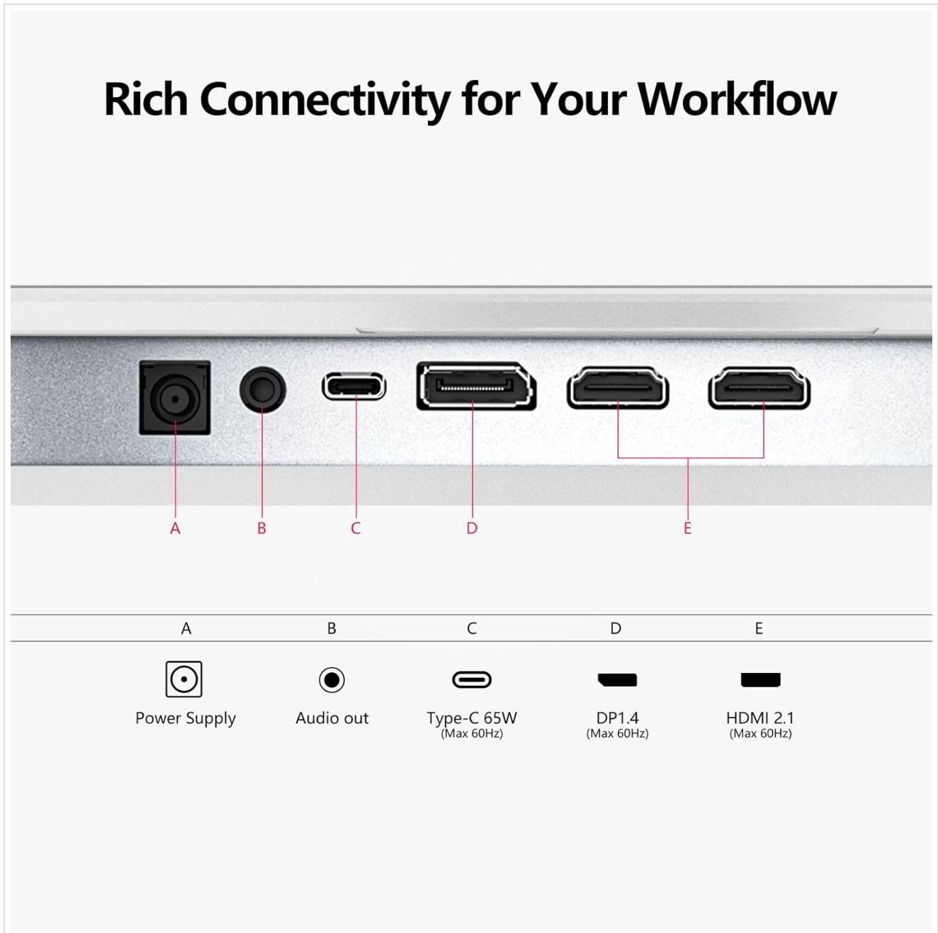
Figure 1: Rear view of the monitor displaying available ports including Power Supply, Audio Out, Type-C (65W), DP1.4, and HDMI 2.1.
