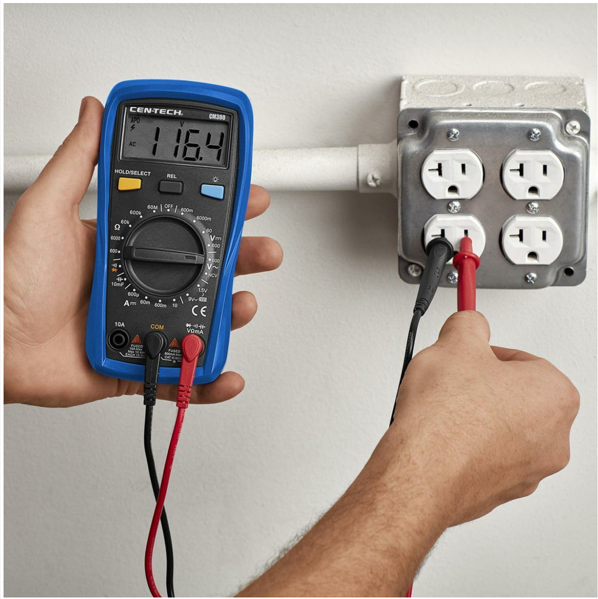
Figure 4.2: An individual using the multimeter to measure the voltage from a standard electrical outlet, demonstrating a practical application of the device.
