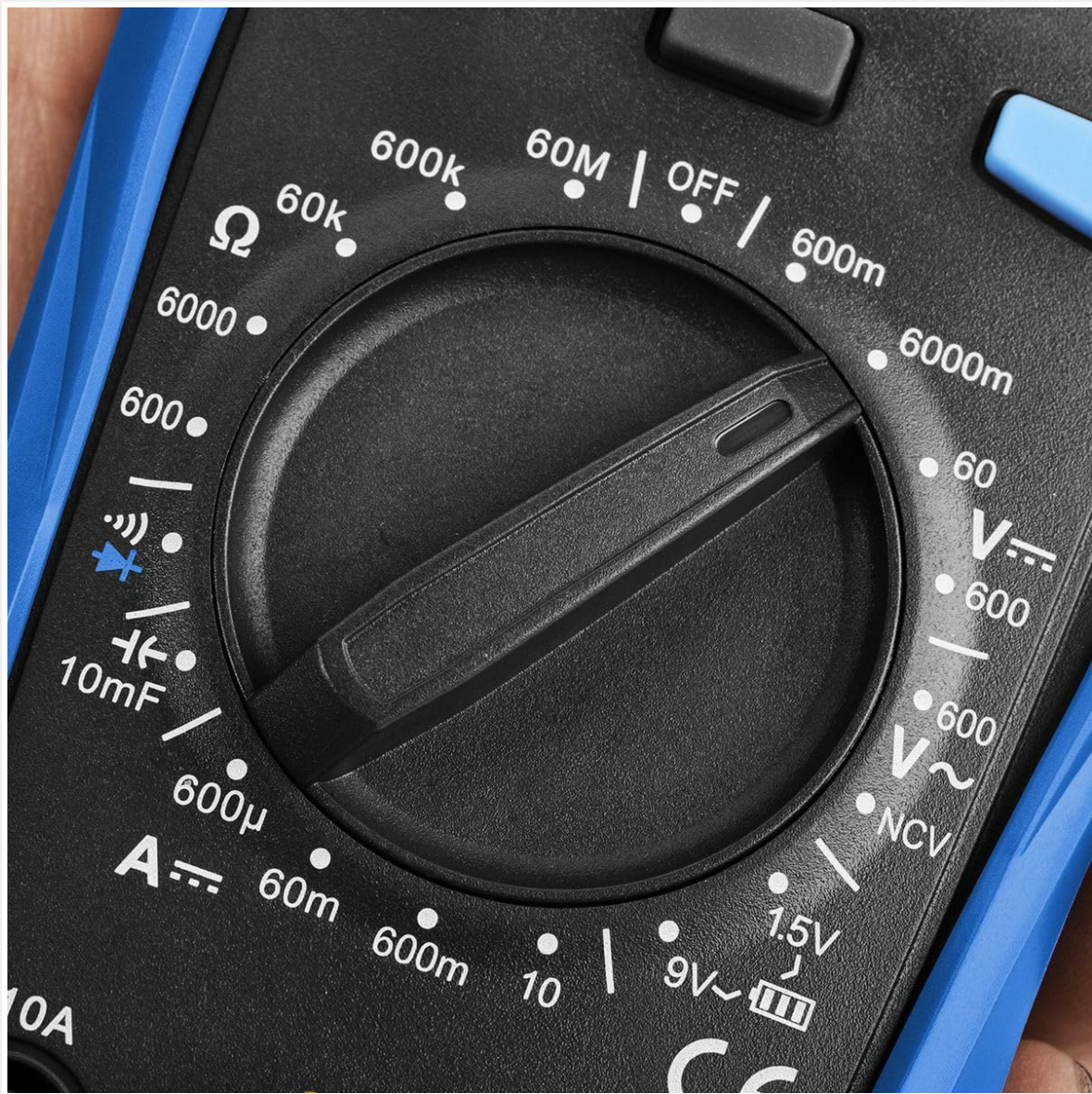
Figure 4.1: A detailed view of the multimeter's rotary dial, showing various measurement functions and ranges, including voltage, resistance, and current settings.
