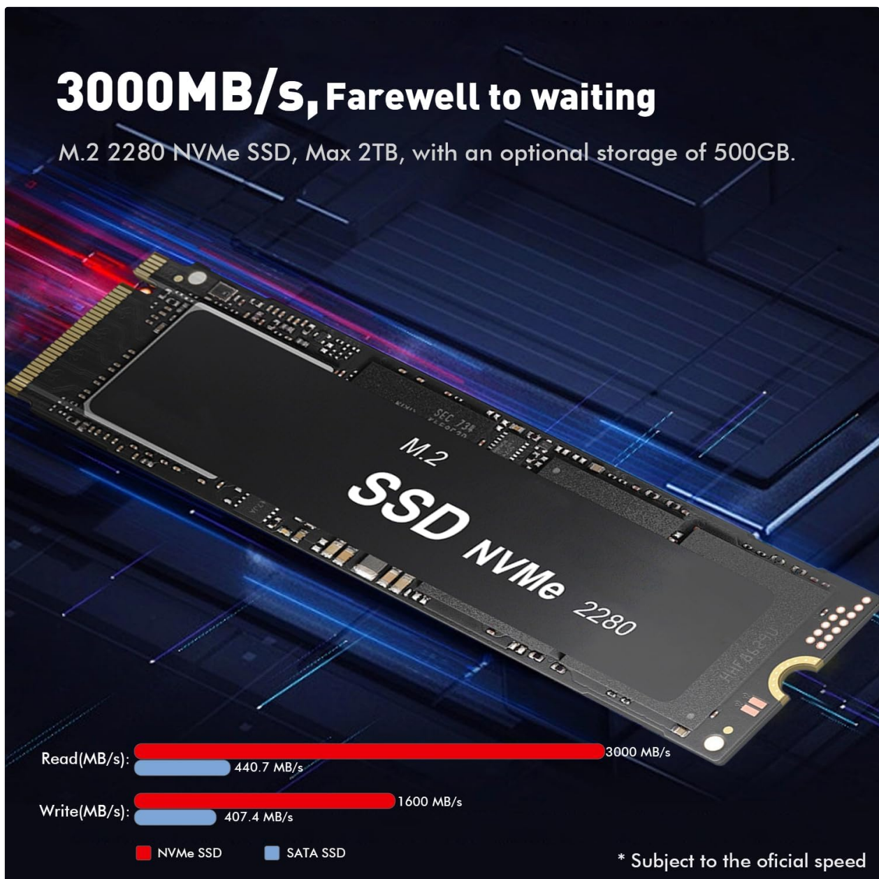
Image 6.2: An M.2 2280 NVMe SSD, highlighting its high read/write speeds and capacity for storage expansion.
