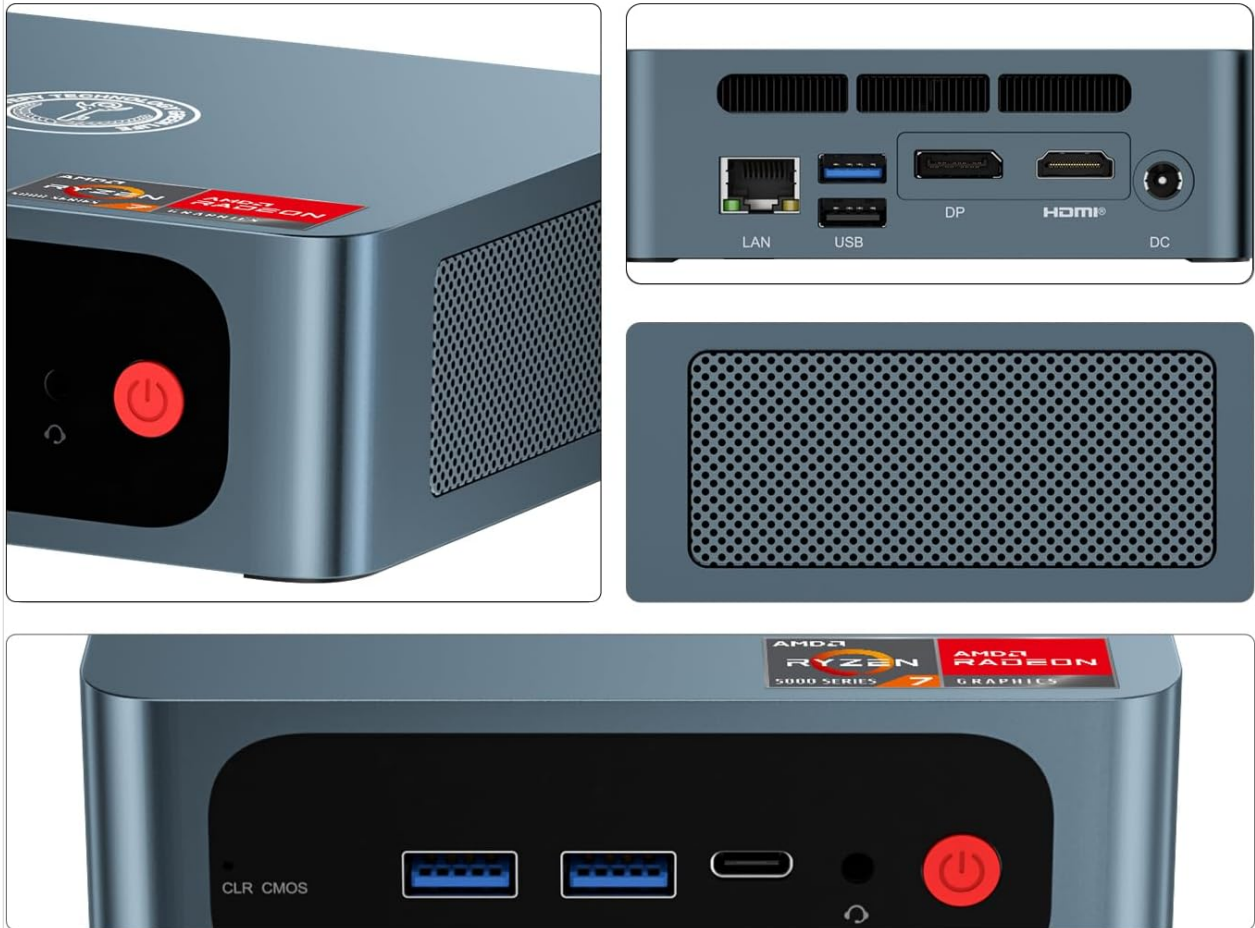
Image 3.1: Detailed view of the TRIGKEY S5 Mini PC's front and rear ports, including USB, HDMI, DisplayPort, and LAN connections.
