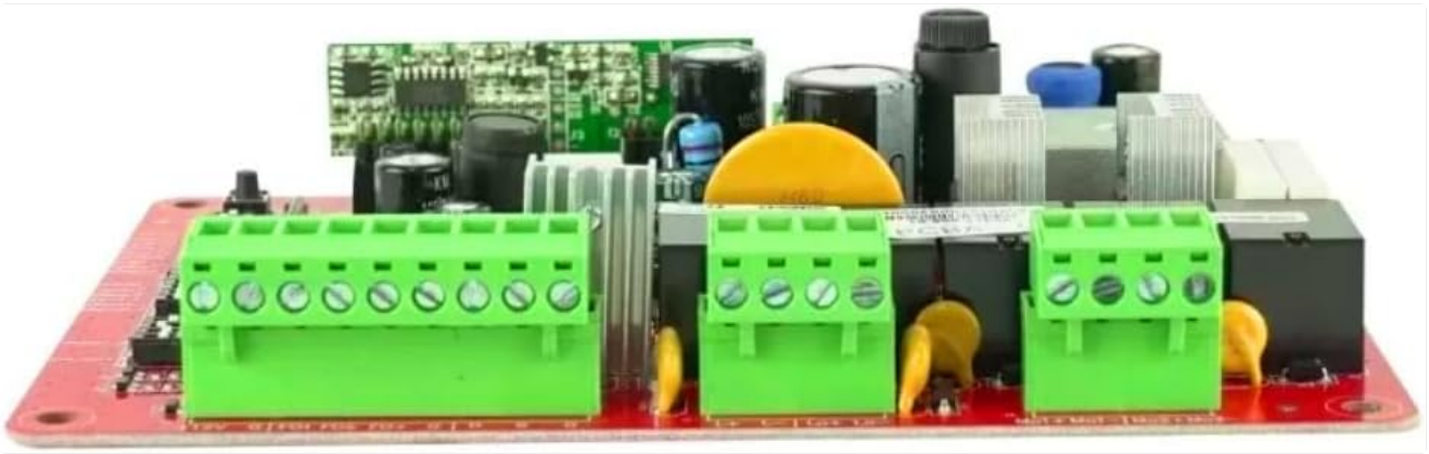
Figure 2: Side view of the electronic board, highlighting the green terminal blocks where external wires are connected. This perspective provides a clearer view of the height of components and the screw terminals for secure wiring.
