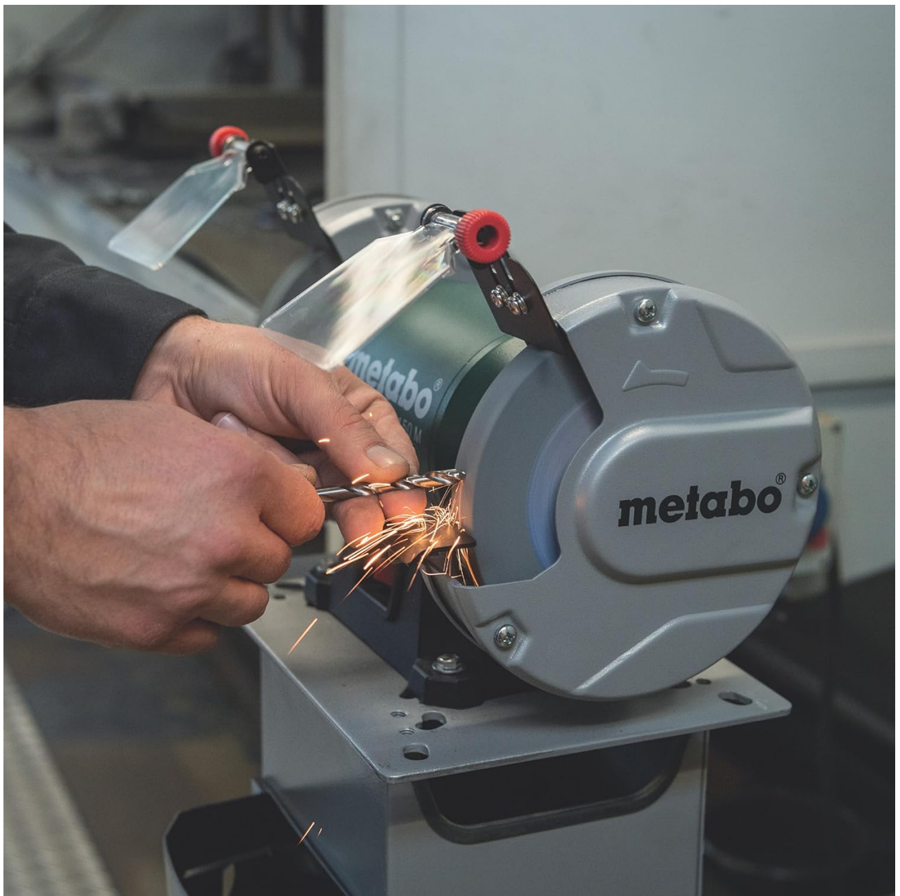
Figure 5.1: The Metabo DS 150 M in use, demonstrating the sharpening of a drill bit with sparks visible, emphasizing the importance of eye protection.
