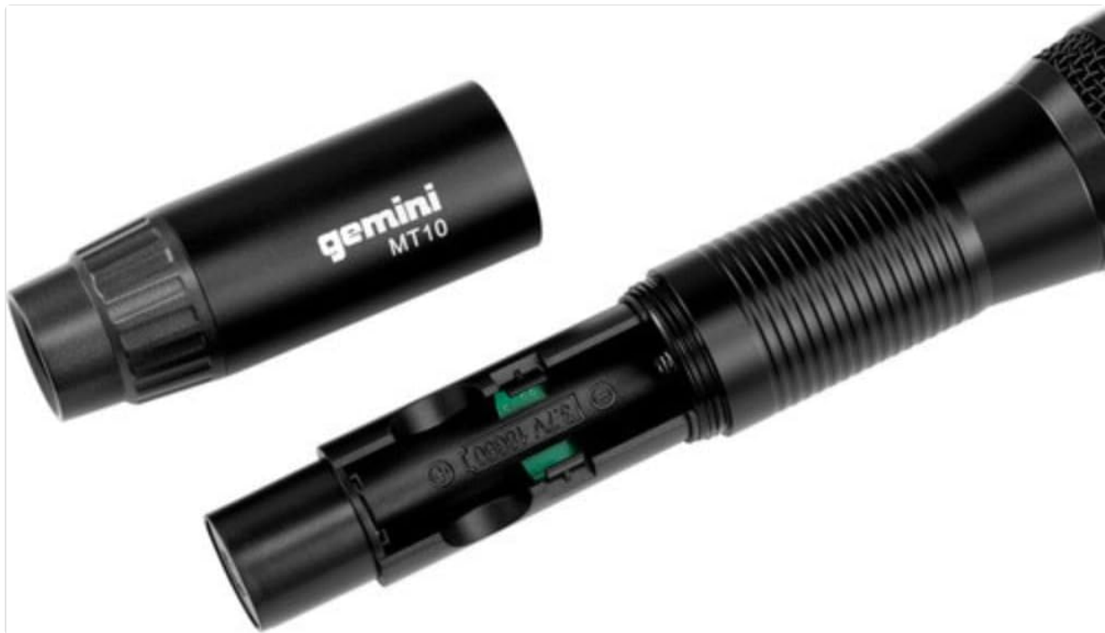
Image 4.3: The microphone with its battery compartment open, revealing the 18650 battery.
