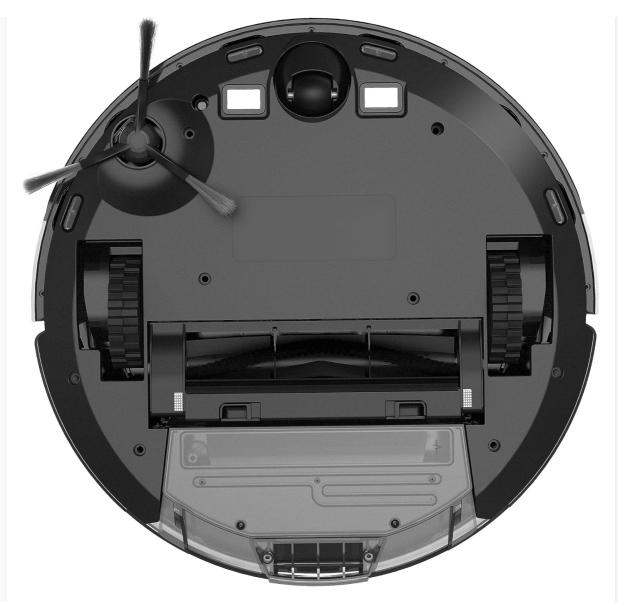
Remove the main brush cover and the main brush. Use the provided cleaning tool to remove hair and debris tangled around the brush. Clean the brush bearings. Reinstall the main brush and cover.
