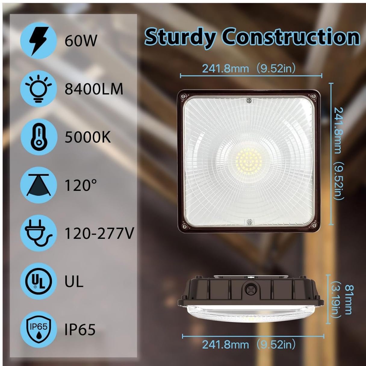
Image 1: Product Dimensions and Key Specifications. This diagram illustrates the physical dimensions of the fixture (9.52 inches L x 9.52 inches W x 3.19 inches H) and highlights its 60W power, 8400LM brightness, 5000K color temperature, 120-277V voltage, UL certification, and IP65 rating.
