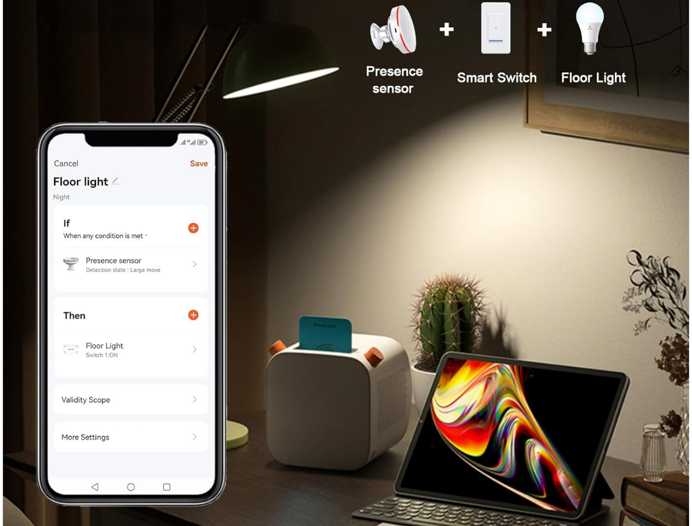
Image: A smartphone screen illustrating the "Smart Linkage Scenes" feature within the app. It shows a rule where detecting a "large move" by the presence sensor at night automatically triggers a floor light to turn on, demonstrating integration with smart switches and lighting.
