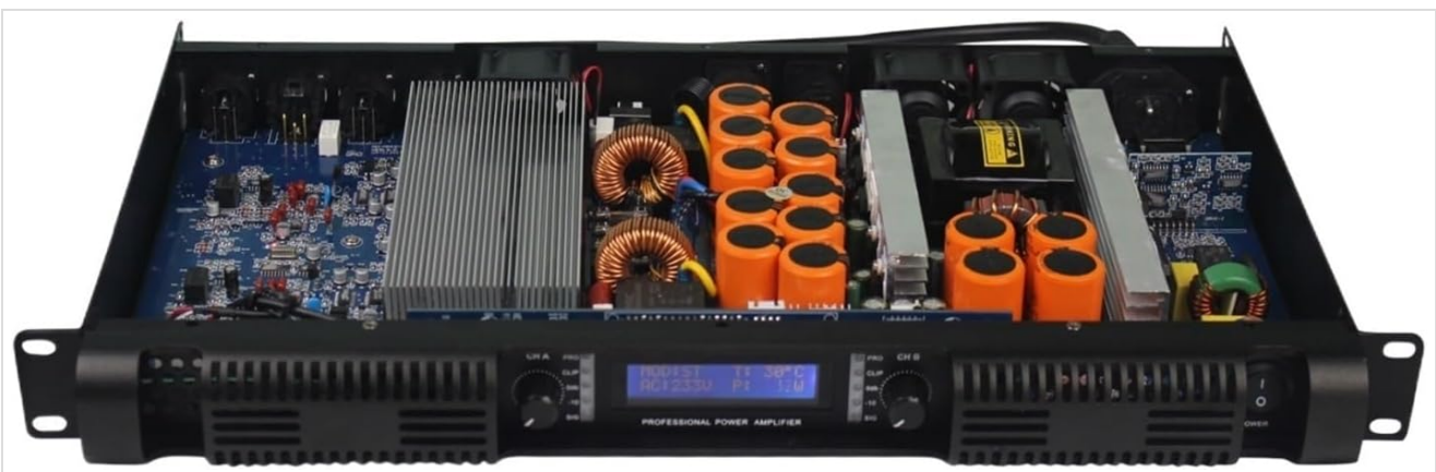
Figure 3.4: Internal Components View. This image provides a look inside the HEXEH GAP-XS1000, revealing the circuit board, large capacitors, transformers, and heat sinks, illustrating the robust internal construction designed for powerful and stable operation.
