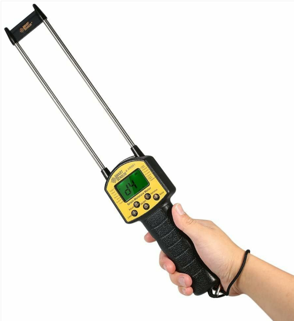
Figure 3.1: The Smart Sensor AR991 Digital Grain Moisture Meter in use, demonstrating its ergonomic design and clear LCD display.
